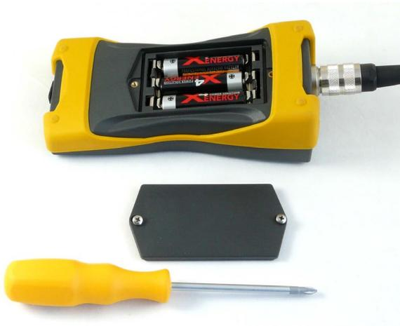
The device will be delivered with batteries mounted. To exchange the batteries open the battery compartment with a Philips screw driver. Remove the batteries if they might not be used for a very long time e.g. than powering by USB only.
