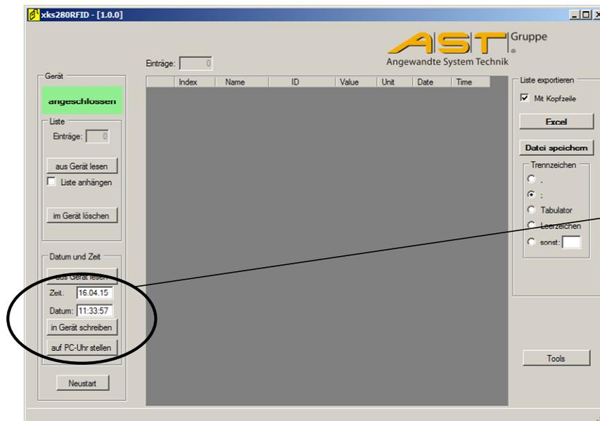
Figure 8: Software “xks280”: Setting the clock on the Data Logger
