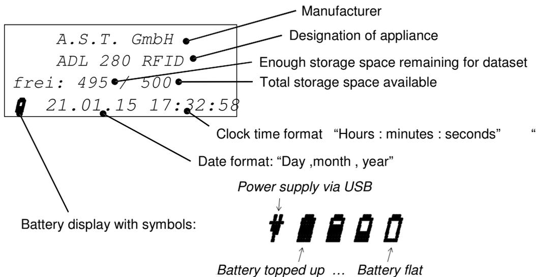
Figure 3: Display after appliance has been switched on
