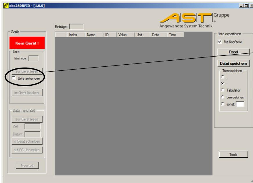
Figure 5: Software "xks280": Continuation of an existing list
