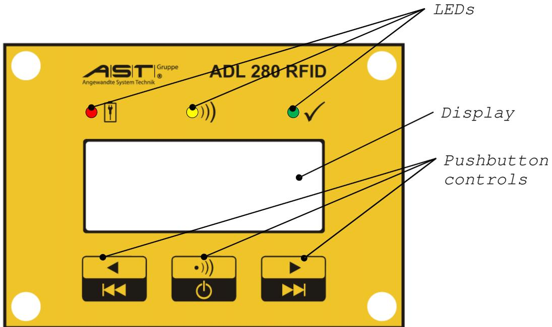
Figure 2: Operating controls and display functions on the Data Logger
