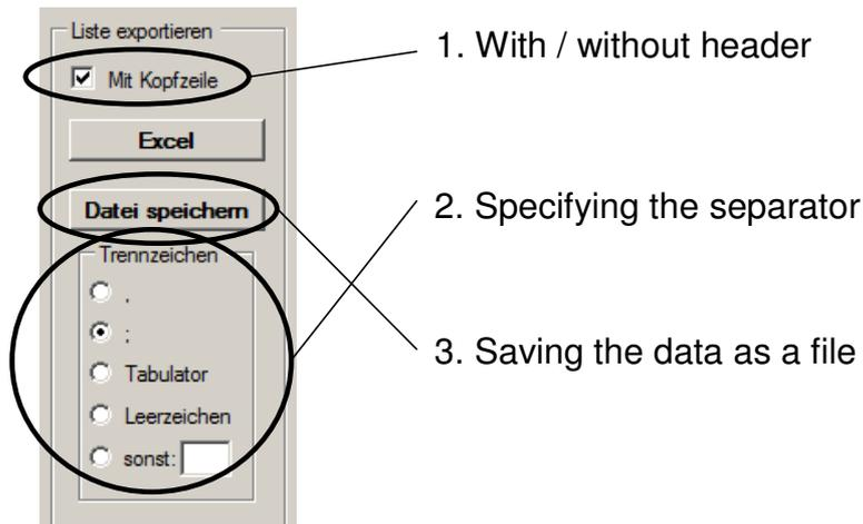
Figure 7: Software “xks280”: Options for saving the list as a file
