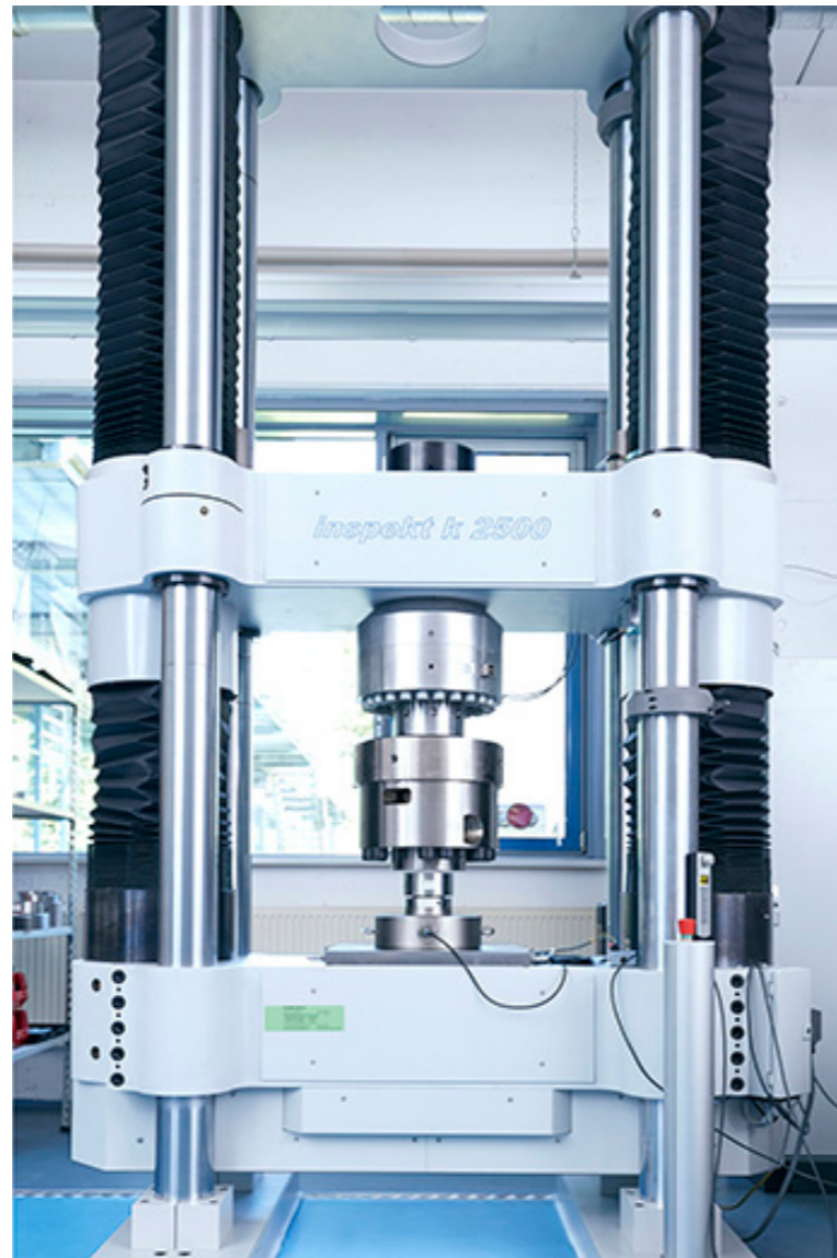
We do DAkkS calibrations from 500N up to the high load range from 2MN..
