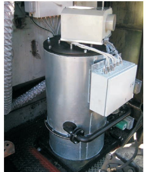
Installation example 50 kW ASTop-Idle system with integrated TEG modules on an EMD GP38
